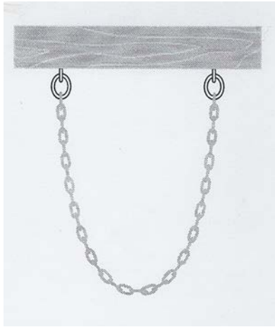
Fig 2: The catenary curve
