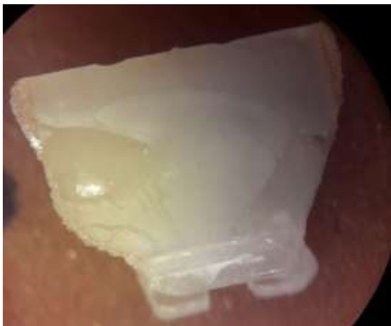
Fig. 5. A debonded sample with ceramic bracket cracks.
