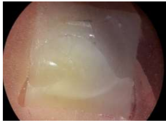
Fig. 6. A debonded sample with composite block cracks.
