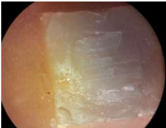
Fig. 4. A debonded sample with ceramic bracket cracks.
