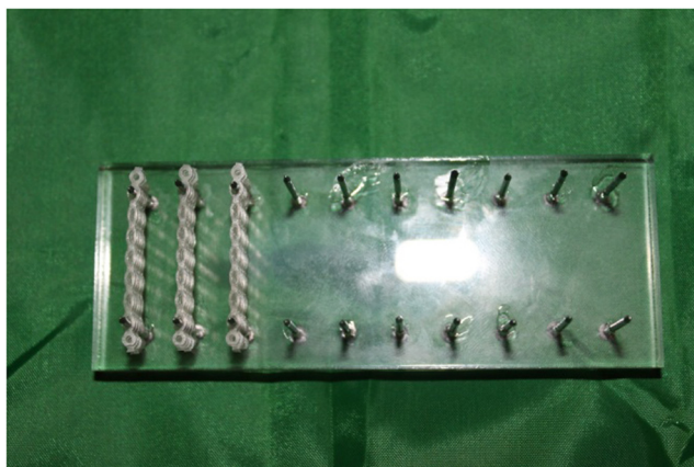
Fig. 1 – Fabricated device made of stainless steel rods to hold the chains stretched at the length of 24mm.
