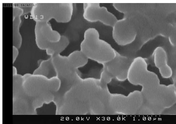
Fig. 1. Nano chitosan under scanning electron microscope (magnification: 30.0 KX).
