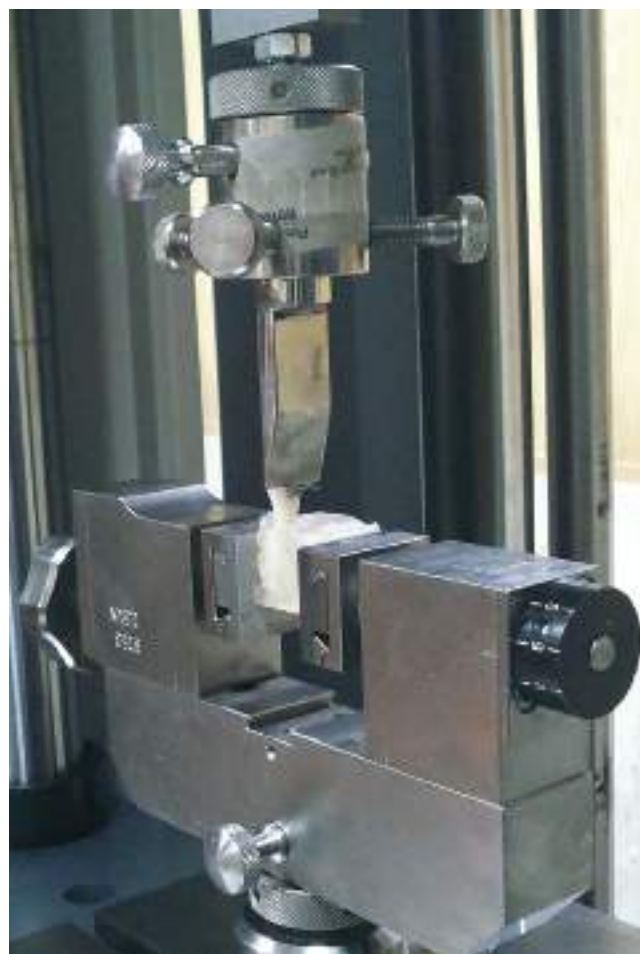
Figure 1 - A 0.6-mm metal blade was used to apply shear force to the composite interface.
