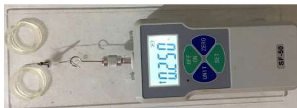
Figure 2. The force was measured using a digital force gauge.
