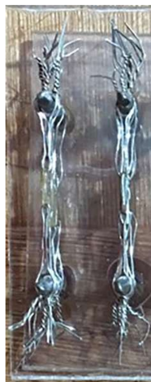
Figure 1. The two types of active tiebacks were stretched so that they exerted 250 gr force initially at the 24 mm extension
